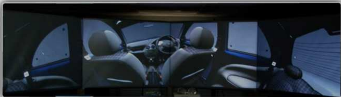
Surface: A 32 foot wide projected power wall display, driven by four networked computers
